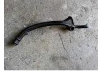
2. The 2 smaller locating tabs will need to be removed so the part will fit inside the new SpeedyMoto center cover. You can do this with a pair of dykes.
