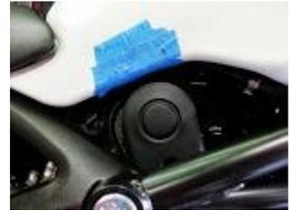
2. Before removing the stock belt covers, find the plastic guard holding the wiring harness behind the exhaust, clip the zip tie, so this part can be easily removed (BE CAREFUL NOT TO DROP THE SPACER).
