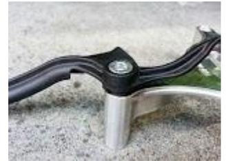
4. Install new SpeedyMoto center cover first with the stock wiring harness guard and use the supplied hardware and a drop of blue Loctite on each bolt. ATTENTION! Be sure to capture the wiring harness with the guard so it does not touch the exhaust or interfere with the belts. Use the supplies tip ties to secure the wiring harness to the guard.
