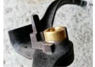
3. File or shave the inside of the large single locating tab so the guard will fit into the SpeedyMoto cover. This can be done with a small file or a sharp blade.
